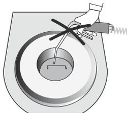
This product contains ceramic fibres and may release fibre dust. Do not use compressed air on the furnace, thus distributing the dust in the environment, and observe the additional notes on page 11.
