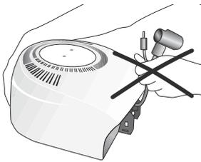
Do not carry the furnace head by the cables, since the cables and connections may be damaged.
