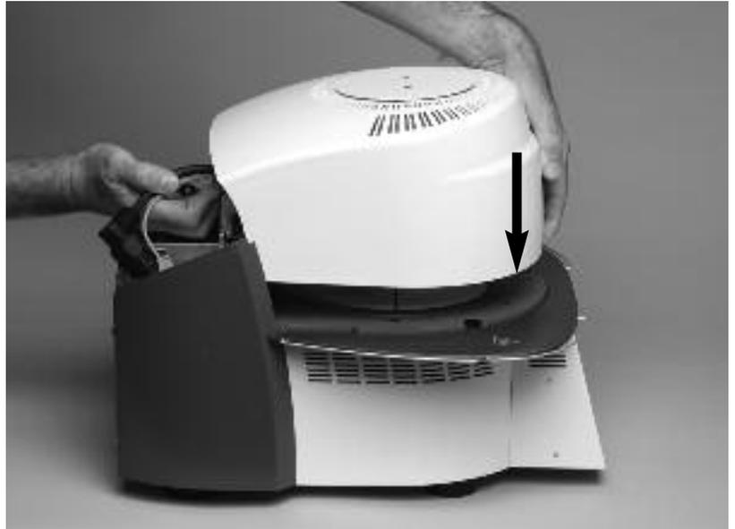
Ensure that the furnace head mounting mark (41) is aligned with the furnace base mounting mark (42).
