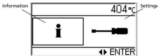
The cursor position (frame around the symbol) can be changed by means of the cursor keys. To view the required Settings or Information, press the Enter key.
