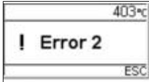
The furnace continuously checks all functions during operation. If an error is detected, the respective error message is displayed.
