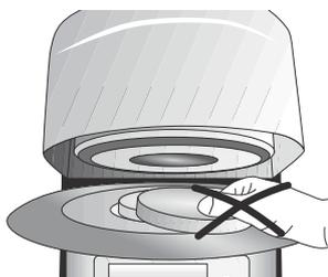
Never place objects in the firing chamber by hand, since there is a burn hazard. Always use the tongs (accessories) supplied for this purpose. Never touch the hot surface of the furnace head, as there is a burn hazard. Please also refer to the warnings on the furnace.
