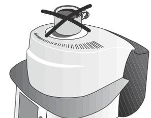
Foreign objects must not be placed on the furnace head or the air vents. Make sure that no liquids or other foreign objects enter the air vents, since this may result in an electrical shock.
