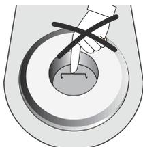
Do not touch the thermocouple and the quartz tube in the firing chamber. Avoid contact with the skin (grease contamination), as the parts will be prematurely damaged.
