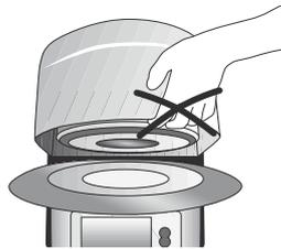
The furnace has an electric drive and must be operated by means of the electronic controls. Never open the furnace head by hand, since the mechanism will be damaged.
