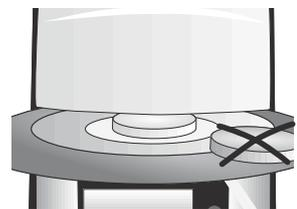
Firing trays must not be placed in the area surrounding the firing table, since this will obstruct the closing of the furnace head.
